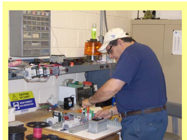
Treatment and Pumping Operator fabricating control panel for remote operation of pumping station
